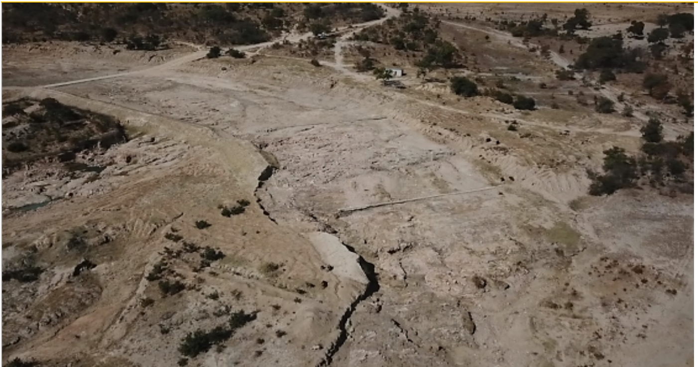
Spillway channel showing 2018 breakthrough channel and 2019 damage
