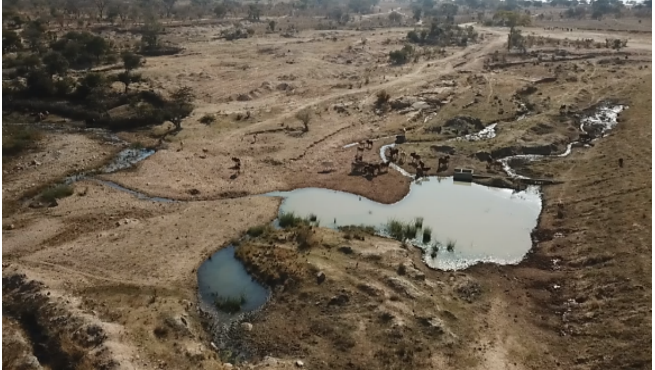
Figure 18 Disturbed, eroded areas and former borrow sites downstream of the dam
